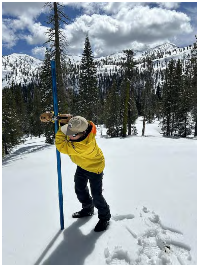
Ranger Sam Clairmont takes a core sample from the Gray Rocks snow survey site, conducted monthly by Forest Service employees. Important data such as height of snow and water content is derived from measurements. This information is essential for state water allocations
